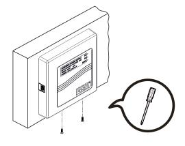
Ease of maintenance: Use the included wrench to remove the bottom screws and cover for routine checks or troubleshooting.
