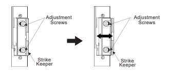
The keeper can be moved horizontally to compensate for installation difficulties such as warped doors. (Maximum adjustable range: 3mm)
