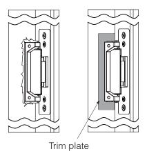
Trim plate is used to cover any imperfections caused while prepping the frame cut out.
