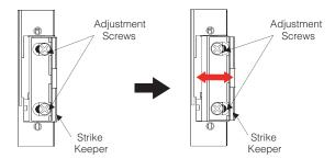
The GK515/515M/525/545 features an **adjustable keeper** that can be moved horizontally to compensate for installation difficulties such as warped doors. **(Maximum adjustable range: 3mm)**
