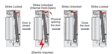
The hold-open function (Internal) enables strike to become unlocked after single electric impulse. The electric strike is open until physical opening the door, then the latch is coming back to standard position (closed). Internal hold-open has no extending switch and does not have to be adjusted to the door latch.
