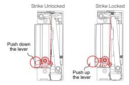
The GK520/525 features a mechanical lever that can be activated to keep the strike opened until pushed back manually.
