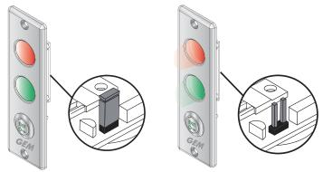
Select Solid or Flashing LED with jumper setting
