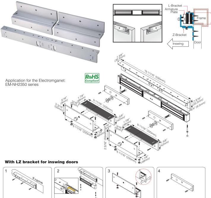
Install L bracket on the door frame. Make sure the door may be opened / bracket with fixing screws. closed.
