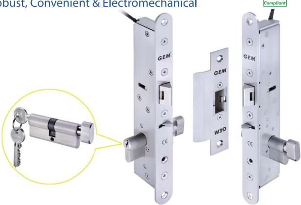
The ML-655M electric lock is a high performance lock designed for single action swing doors. Featuring a double action latchbolt and left/right side adjustable deadlatch tip, the ML-655M allows deadlocking automatically when the door is closed to be secured for ease of use and convenience. The ML-655M can be controlled by card readers/keypads and connected to automatic swing door operators for an integraed access control solution.
