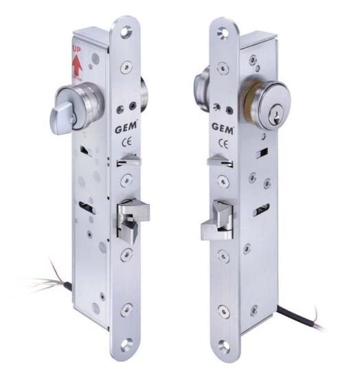
The ML-805M electric lock is a high performance lock designed for single action swing doors. Featuring a double action latchbolt and left/right side adjustable deadlatch tip, the ML-805M allows deadlocking automatically when the door is closed to be secured for ease of use and convenience. The ML-805M can be controlled by card readers/keypads and connected to automatic swing door operators for an integraed access control solution.
