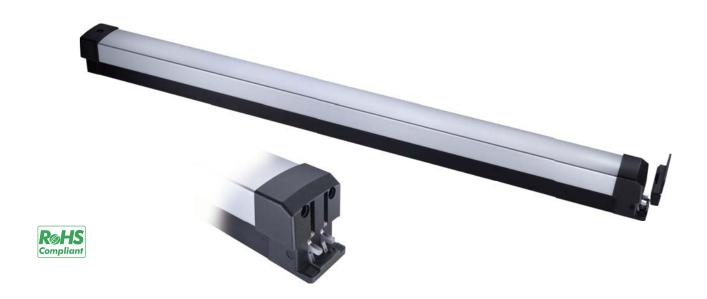
PBH-100 series electromechanical push bars are electrified exit devices designed to work with access control as means of locking mechanism. On exit, simply depress the push bar to open the door. It is recommended to pair with key cylinders or access control devices on the exterior.
