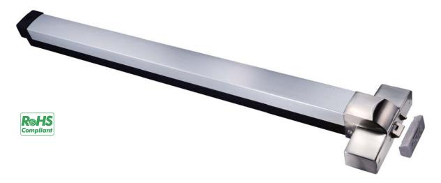
The PBH-350 Series Electromechanical Push Bar is designed for use on emergency exit doors. It provides a convenient means of escape by simply pushing on a horizontal bar fitted across the width of a door. It also features preload release capability that overcomes door preload problems, such as air-conditioning pressure, changes in the weather, warped doors or doors with weather stripping.
