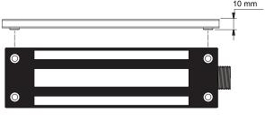
Thickness of 10 mm with enhanced sturdiness to secure the magnetic lock
