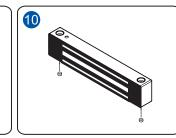
The rubber washer makes the armature plate adjustable in order to reach the utmost to align combination with magnet lock.
