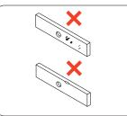
Make sure the contact area of the electromagnet lock and the armature plate are clean or the bond sensor output function will not work.
