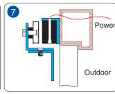
Test the tightness and adjust the Z bracket to fit the door.
