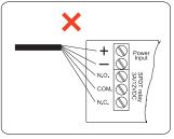
Do not apply power wires and signal wires in the same cable or conduit.
