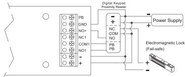
Using the output from digital keypad/proximity reader to control PBA-860LD (Dry Contact).
