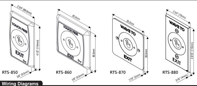
The RTS series wave sense infrared exit device includes one set of output contacts NC/NO/COM. It can be connected to an access control device (e.g. keypads or proximity readers) as shown in Figure A or can directly control electric locks (e.g. maglocks or electric strikes) as shown in Figure B.
