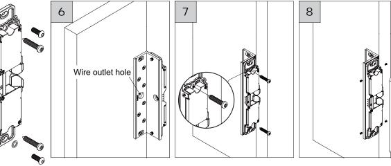
Drill a 6mm wire outlet hole. Secure the rim mount strike to the bracket as indicated.
