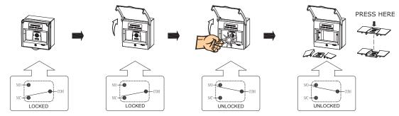
Open the clear plastic cover. Press harder to break the plastic glass so that the switch will change status from NC to NO, triggering the connected device.
