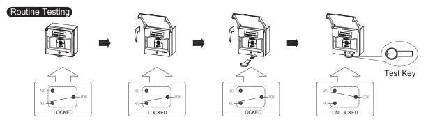
Open the clear plastic cover. Insert the test key into the hole so that the plastic glass will tilt to one side and the switch will then change status from NC to NO. Remove the test key so that the switch reverts back to NC status.
