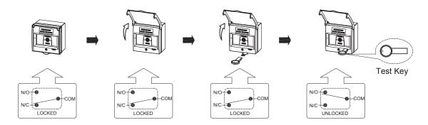
Take the clear cover off. Insert test key into the test hole, so that plastic glass will tilt to one side, switch contact will then change from NC to NO status. When completed, remove the test key, so that it reverses back to the NC status.
