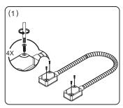
Remove the security screws using the enclosed tool.
