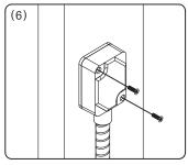
Connect the wire to each end of the Mount the head covers and tighten the screws.
