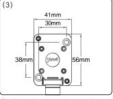
Position the two end caps where you plan to mount them and mark the holes on the door and frame.
