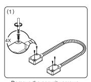
Remove the security screws using the enclosed tool.
