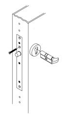
Use 45x45mm tighten the cylinder
