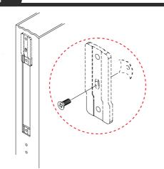
Position screws for fasten Fixing Lugs
