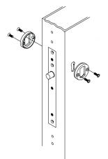
Insert electric dropbolt into position, attach to Fixing Lugs and base
