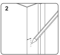
Mark the position of the latch bolt on the door frame as shown in the figure.
