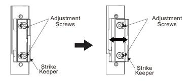
The strike keeper can be adjusted horizontally to account for various installation anomalies. To adjust the keeper, loosen the adjustment screws, move the keeper horizontally as needed, and retighten the adjustment screws.
