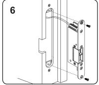
Connect the wires and install the strike.
