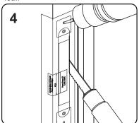
Drill and cut the frame according to the template.
