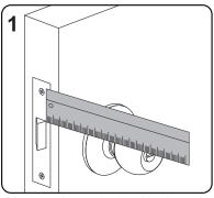
Measure the vertical and horizontal position of the latch bolt on the door leaf.
