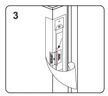
Mount the supplied template and align to the marked line.
