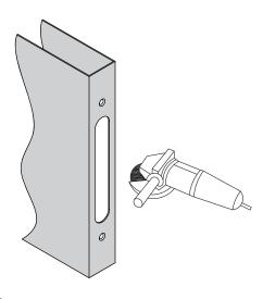
2c. Check if the WLP-100 fits well in the cutout and use the file if necessary.
